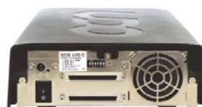
Rear View - UDO Desktop Drive (SCSI interface)
